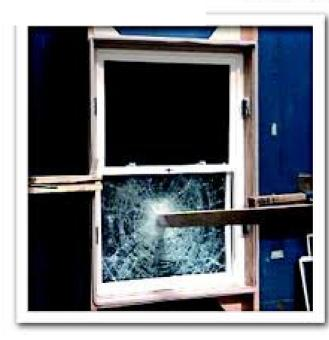
Florida tests hurricane products by changing wind tunnel pressures on them repeatedly, and by shooting large pieces of wood out of a cannon at high speeds (left). The resulting product test score is the FL# (State Product Approval Number); for us, products should be rated at 150 – 180 mph windspeed. Keep in mind that these test condiitons are not nearly as powerful as thewind, rain and debris damage 18 done during a hurricane.
